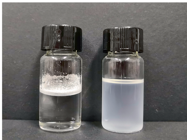
Fig. 4. Photograph of the dispersion state of PMSQ in water (left) and toluene (right).
